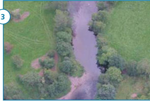
3 Silt erosion, with downstream deposition and formation of an island with implications for alterations in flow regime with possible flooding or further erosion during high flows.
